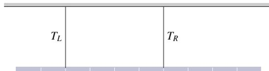
A horizontal uniform meter stick of weight  $W$  hangs from vertical strings at the 20-cm and 60-cm lines. What are both tensions,  $T_L$  and  $T_R$ ?
