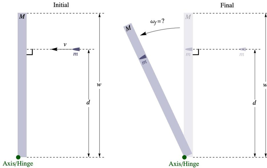
A bullet of mass  $m$  is shot at speed  $v$  toward a door. The bullet's velocity is perpendicular to the door and it hits the door at a distance  $d$  from the door's hinge. The door has mass  $M$ , height  $h$  and width  $w$ ; assume that it swings without friction about the hinge. If the door is initially at rest then what is its angular velocity after the bullet embeds in it.
