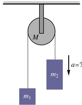
In chapter D we solved Atwood's machine with an ideal pulley. Recall that an ideal pulley was frictionless and light, where light means that the pulley's mass is small compared to the other masses in the system. Now we will consider a pulley with mass; it will still be frictionless. With an ideal pulley the tension on both sides is the same. Here, with a massive pulley the tensions on either side are different. The different tensions are responsible for the angular acceleration of the pulley.
