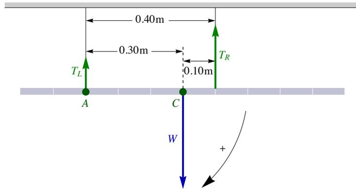
We may choose the axis anywhere. Any force that acts at the origin produces no torque. If we choose the axis to be when an unknown acts then the torque equation will not involve that unknown. We will choose the axis labeled  $A$  where  $T_L$  acts. Choosing clockwise as our positive sense of rotation we can write the torque equation and can solve for  $T_R$
