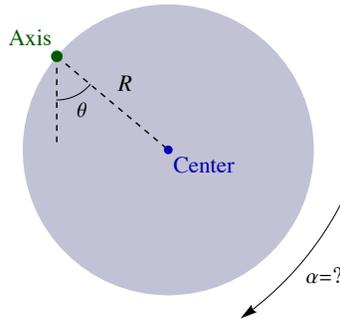
A uniform disk of radius  $R$  swings without friction about a perpendicular axis through its rim. What is its angular acceleration as it swings through a position where the center is at an angle of  $\theta$  from vertical, as shown?
