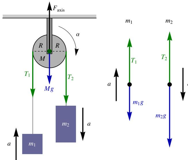
Applying the second law to the hanging masses gives a pair of equations. Here we choose the directions of the accelerations as positive.
