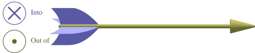
Figure: The convention we use to represent the third dimension relative to some two-dimensional figure is to use a dot to represent "out of" and an x to represent "into". A useful way to remember this is with an arrow; if it points at you it is a dot and away an x.
