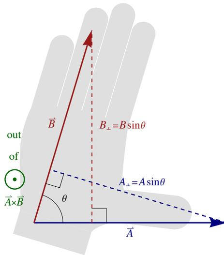
To find the direction of the cross product  $\vec{A} \times \vec{B}$ , put the thumb of your right hand in the direction of the first entry  $\vec{A}$  and your fingers in the direction of the second entry  $\vec{B}$ . The palm of your right hand points in the direction of the cross product.
