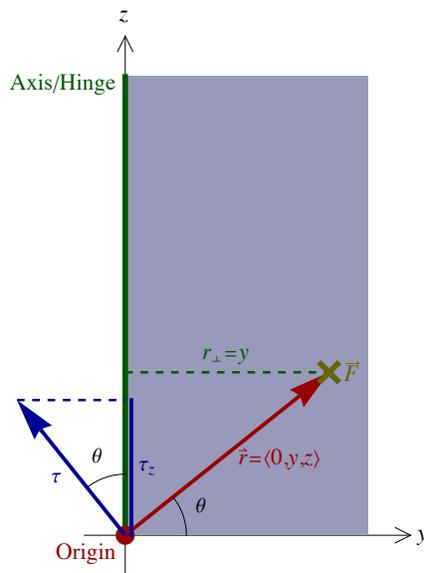
Consider a door in the  $yz$ -plane with the hinge as the axis in the  $z$ -direction. The origin is at the base of the door. A force of magnitude  $F$  pushes into the door, in the negative- $x$  direction.
