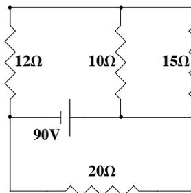
Complete the table below with the voltage across, the current through and the total power dissipated in each resistor.
